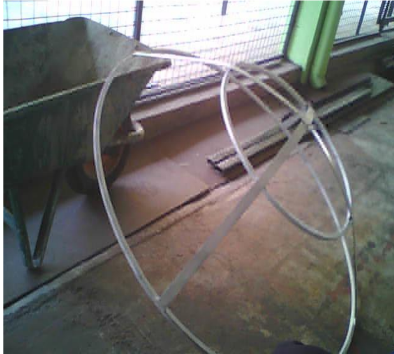
Figure 3.3 The parabolic cage after finishing process.
