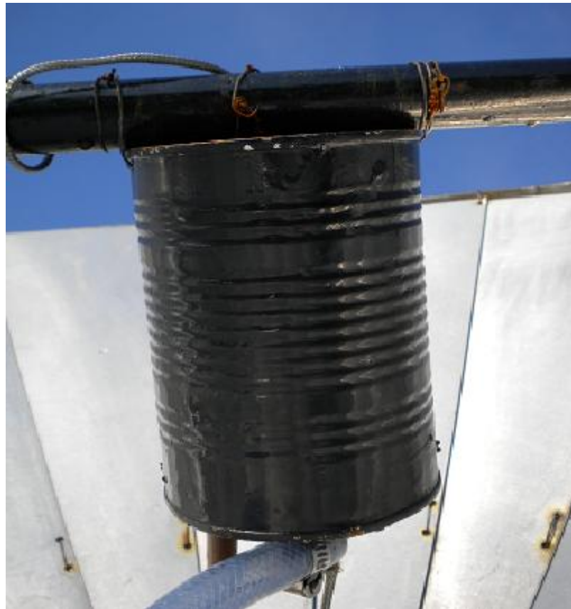
Figure 3.6: Black body solar heat absorber
