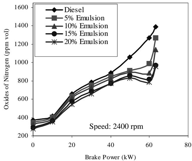
Figure 8 Oxides of nitrogen Vs Brake Power
