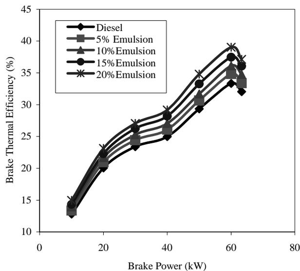
Figure 4 Break Thermal Efficiency Vs Brake Power
