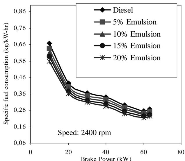
Figure 10 Specific fuel consumption Vs Brake Power using water diesel emulsion by considering diesel as total fuel.
