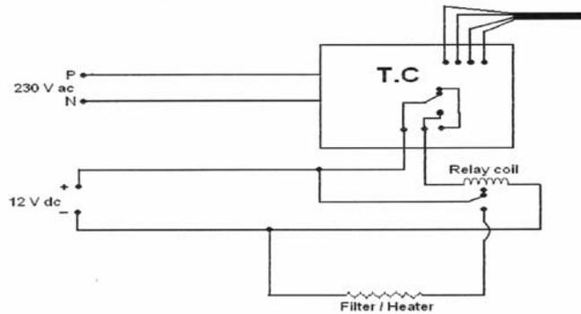
Figure 3 Temperature Controller Circuit of Fuel Management System
