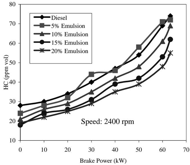
Figure 5 HC Vs Brake Power
