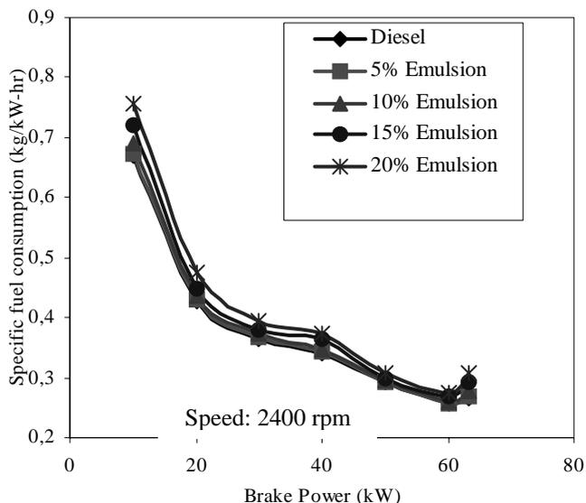
Figure 9 Specific fuel consumption Vs Brake Power using water diesel emulsion by considering water + diesel as total fuel.
