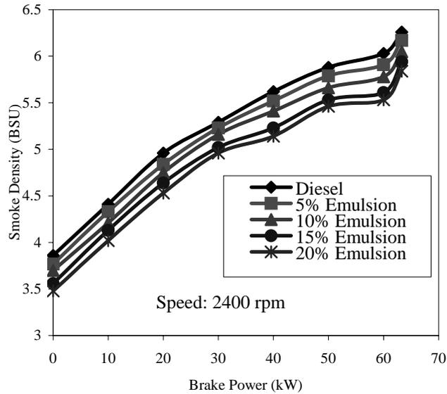
Figure 7 Smoke Density Vs Brake Power
