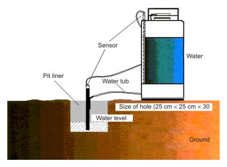
Figure 3 Field infiltration test using Geonor infiltrometer
