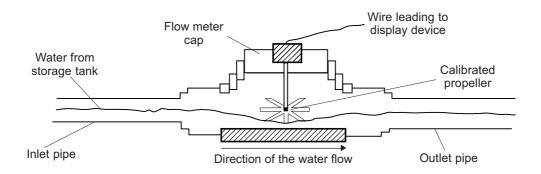
Figure 6 Working concept of a flow water
