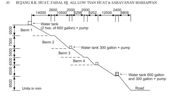
Figure 4 Sectional profile of the cut slope at site B
