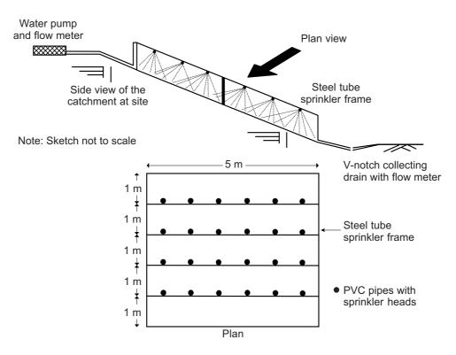
Figure 5 Sprinkling frame and locations of sprinkler heads
