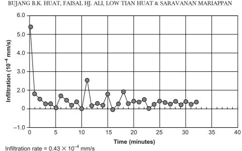
Figure 7 Infiltration rate of granitic residual soil of weathering III (upper boundary) at site A
