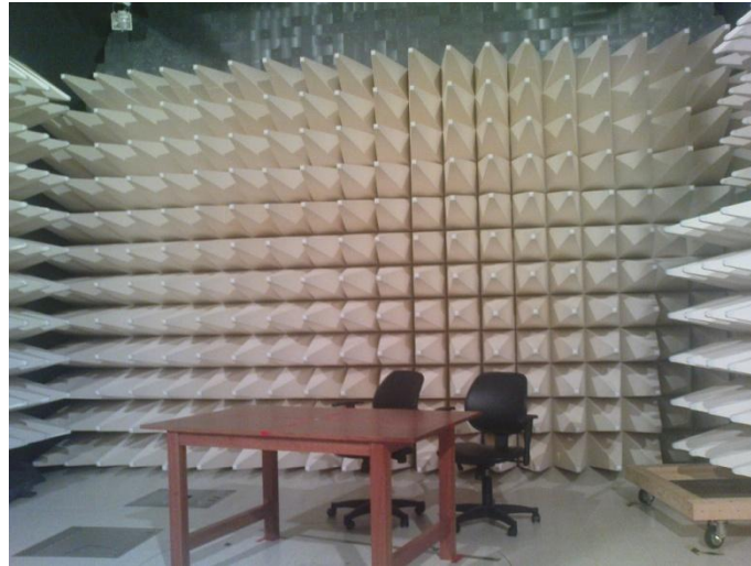
Figure 3.2 Anechoic chamber at the Center of Electromagnetic Compatibility, UTHM.
