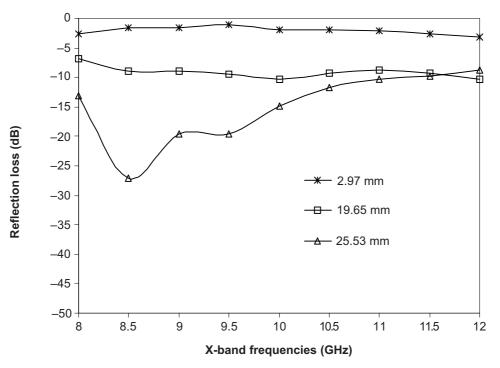
Figure 10 Reflection loss of composites with different thickness of 2.97, 19.65 and 25.53 mm
