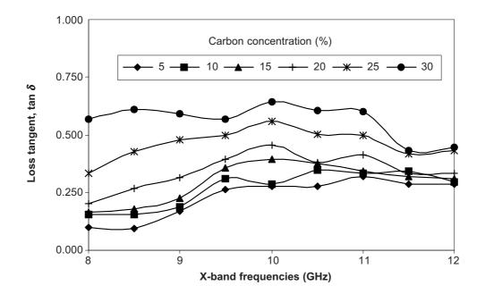
Figure 9 Loss tangent, tan  $\delta$ , at different carbon concentrations (%) in X-band frequencies (Pyrolysed carbon of 800°C)
