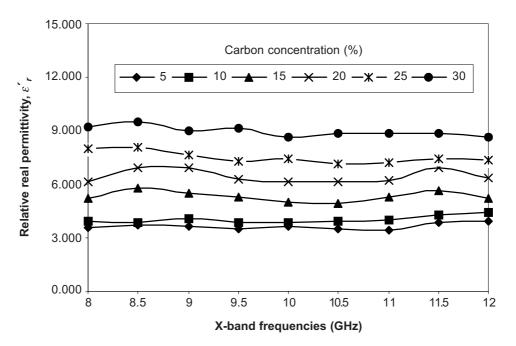
**Figure 6** Relative real permittivity,  $\varepsilon'_r$ , at different carbon concentrations (%) in X-band frequencies (Pyrolysed carbon of 700°C)
