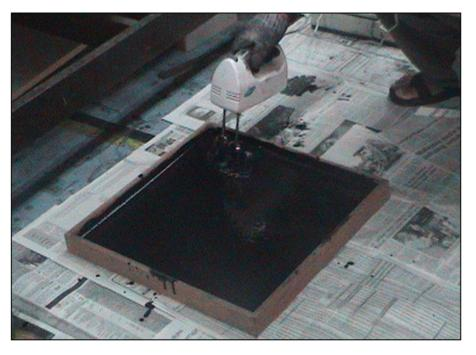
**Figure 2** Samples preparation using  $450 \times 450$  mm wooden mould
