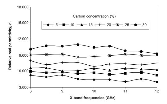
**Figure 8** Relative real permittivity,  $\varepsilon'_r$ , at different carbon concentrations (%) in X-band frequencies (Pyrolysed carbon of 800°C)
