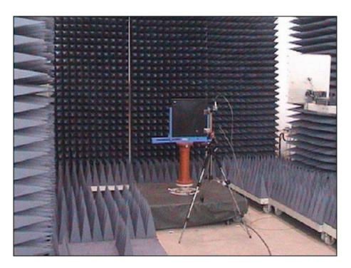
$Figure \ 3 \quad {\rm Free \ space \ reflectivity \ measurement \ set-up}$
