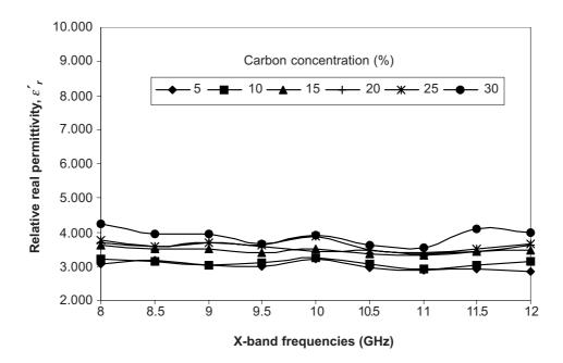
**Figure 4** Relative real permittivity,  $\varepsilon'_r$ , at different carbon concentrations (%) in X-band frequencies (Pyrolysed carbon of 600°C)
