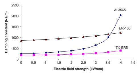
Figure 7 Relationship between electric field strength to the damping constant for nominal damper filled up with particular fluid
