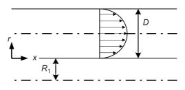
Figure 4 Newtonian fluid velocity profile
