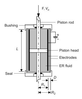
Figure 2 Flow mode ER damper
