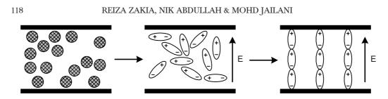
**Figure 3** Schematic illustrations of the ER particles before and after application of an electric field. The two parallel dark lines stand for two electrodes [5]
