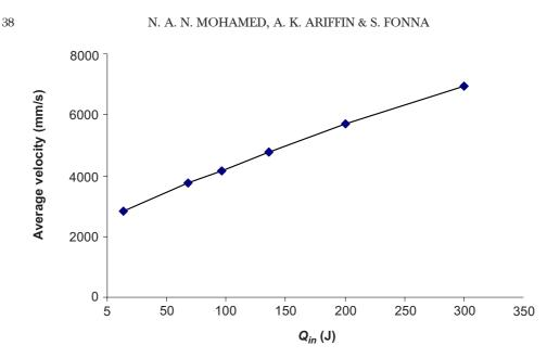
**Figure 11** Piston average velocity versus  $Q_{in}$
