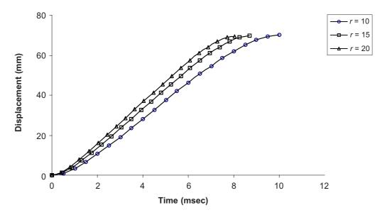
**Figure 7** Piston position versus stroke time for various *r*
