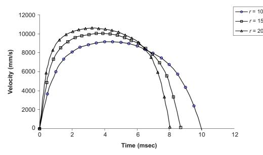
**Figure 8** Piston velocity versus stroke time for various *r*
