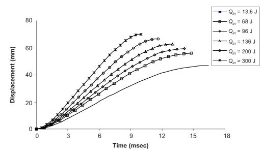
**Figure 4** Piston position versus stroke time for various  $Q_{in}$
