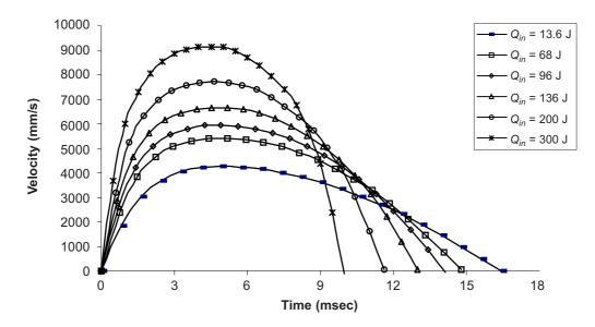
**Figure 5** Piston velocity versus stroke time for various  $Q_{in}$
