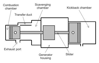
Figure 1 Free piston linear engine model
