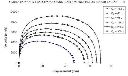
**Figure 6** Piston velocity versus piston position for various  $Q_{in}$
