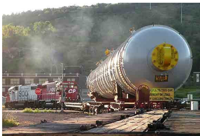
Figure 1.1 A 405 ton, hydro treatment reactor vessel for ConocoPhillips refinery project in Billings (Lakes superior warehousing, 2008).
