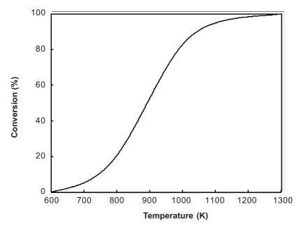
Figure 1 Equilibrium reactant conversions for pure CORM reaction using MTE method
