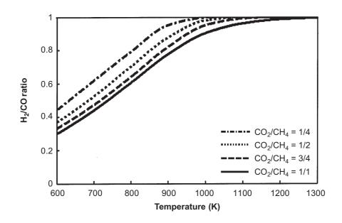
Figure 7 Comparison of  $H_2/CO$  ratios as a function of temperature with different  $CO_2/CH_4$  ratios using LUM method
