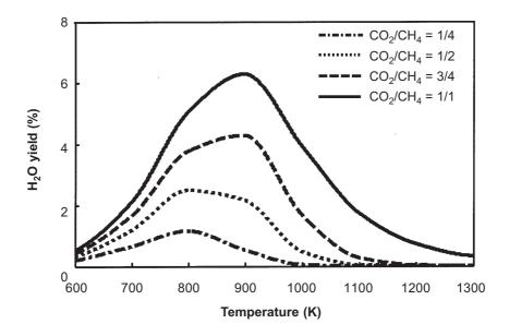
**Figure 6** Comparison of water yields as a function of temperature with different  $CO_2/CH_4$  ratios using LUM method
