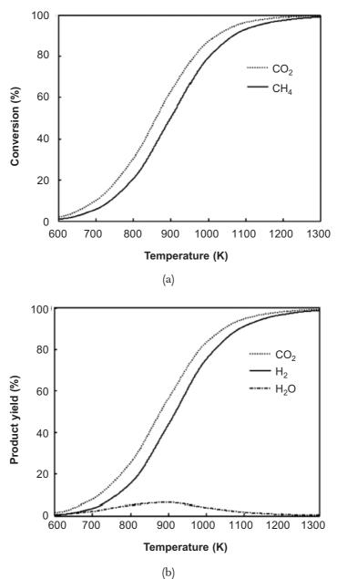
Figure 3 Thermodynamic equilibrium (a) conversions and (b) product yields as a function of temperature using LUM method
