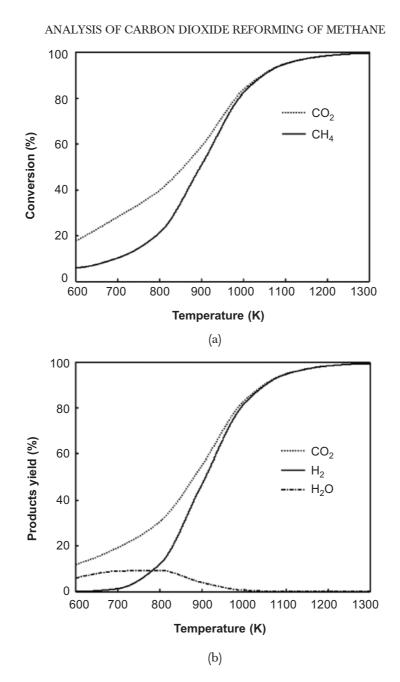
**Figure 2** Thermodynamic equilibrium (a) conversions and (b) products yield for CORM + RWGS reactions using MTE method
