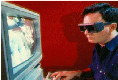
Figure 7.8 An external view of the ARGOS system, which uses a monitor-based configuration (Azuma 1997)
