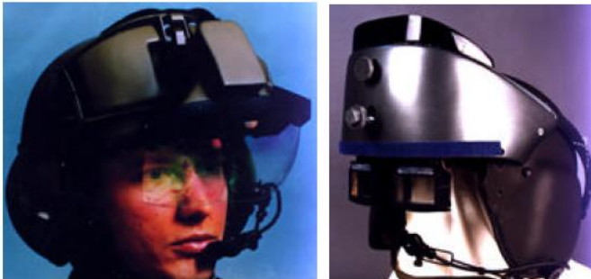
Figure 7.3 Optical see-through HMDs made by Hughes Electronics (Azuma 1997)
