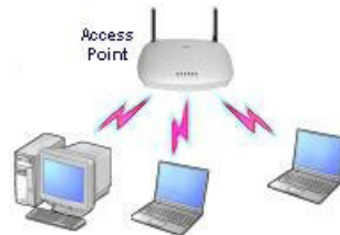
Figure 10.1 WLAN access configuration using Access Point[4]
