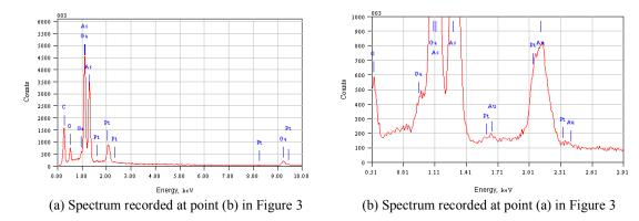
**Figure 4:** EDX spectrum recorded at different positions of the GaAs nanowires. Picture (a) is the spectrum recorded of the GaAs nanowire body. Picture (b) recorded at the tip or head of nanowire.
