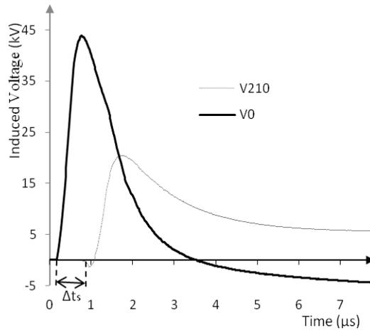
Fig. 7 Induced voltages at both ends with ground lightning strike coordinates of  $(x=50, y=0)$  m.
