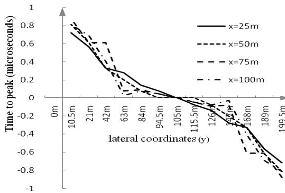
Figure 10: Difference of peak times,  $\Delta t_p = t_{p210} - t_{p0}$
