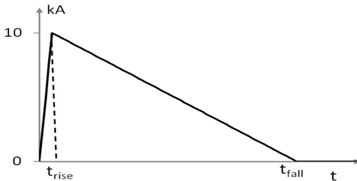
Fig. 2. Ramp type return stroke current
