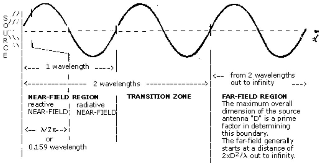
Figure 1 The near and far field in the antenna radiation distances
