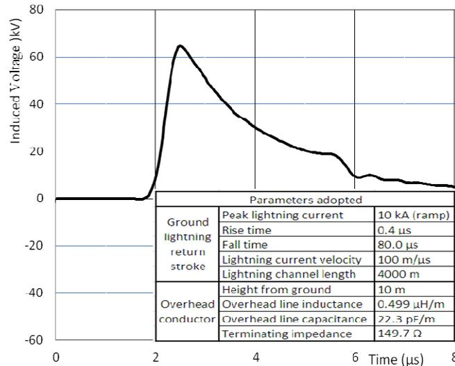
Figure 2: Induced voltages at both ends of an impedance matched 1km overhead conductor due to 10kA peak current ground lightning 50 meters away equidistant to both ends
