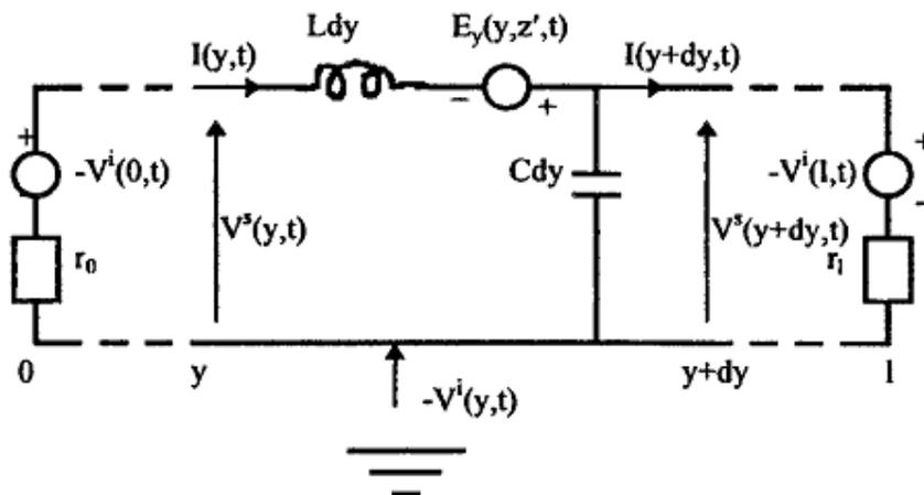
Fig. 3. Differential equivalent circuit for a single-wire lossless overhead conductor
