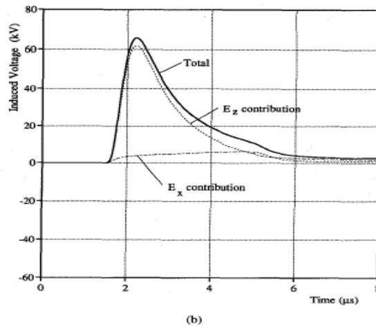
Fig. 3. Induced voltages calculated using vertical and horizontal electric fields with similar parameters to Fig. 2, from Figure 2(b) in [9].
