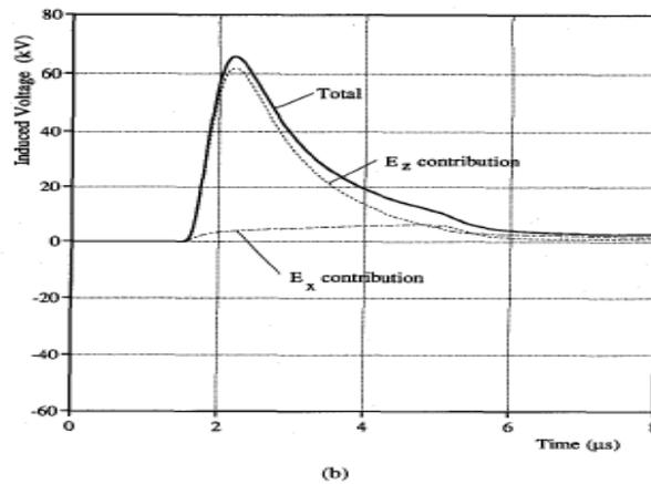
Figure 3: Induced voltages calculated using vertical and horizontal electric fields with similar parameters to Fig. 2, Figure 2(b) in [9]
