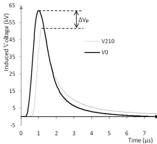
Fig. 8 Induced voltages at both ends with ground lightning strike coordinates of  $(x=50, y=63)$  m.
