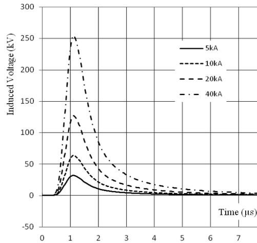
Figure 5: Induced voltages with varying peak GLRS channel base current
