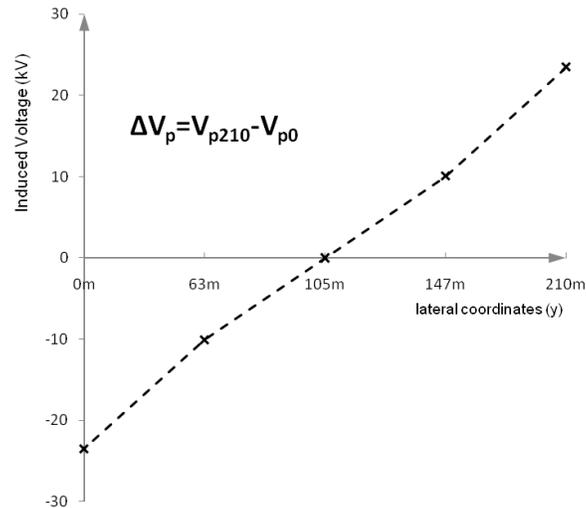
Fig. 12 Difference of peak amplitudes between both ends for the 5 ground lightning strike coordinates.
