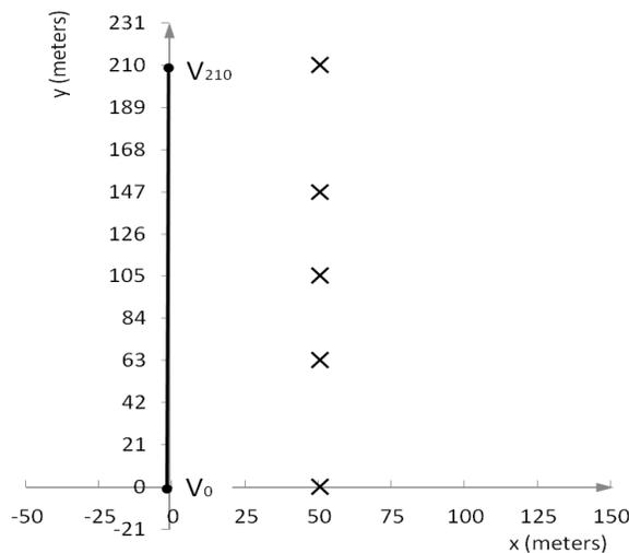
Fig. 6. Plan view of the 10-meter above ground overhead conductor and coordinates of nearby ground lightning strikes
