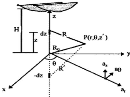
Fig. 1. Geometry of a model nearby lightning used in the vertical and horizontal electric fields computation at a point above ground [7].
