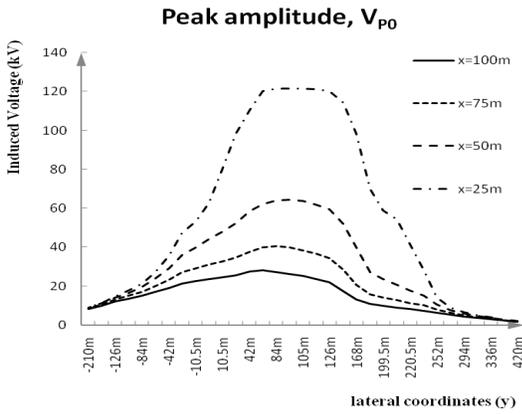
Fig. 6. Peak induced voltages calculated for the first end of the overhead conductor
