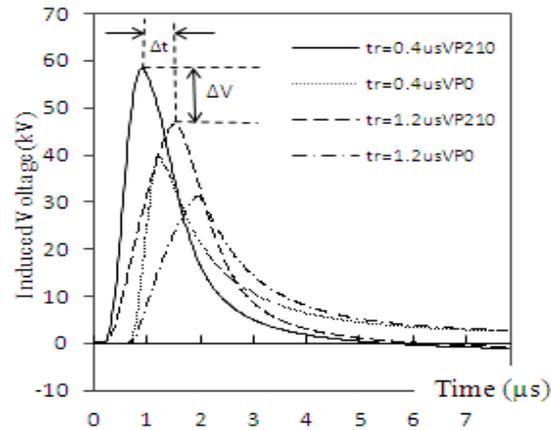
Fig. 5. Induced voltages at both ends with different rise times, indicating the difference of voltage peaks and time to peak.
