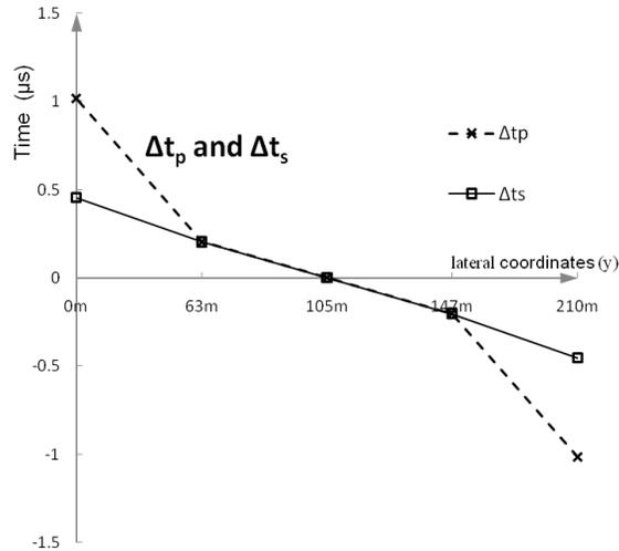
Fig. 13. Difference of start and peak times between both ends for the 5 ground lightning strike coordinates.
