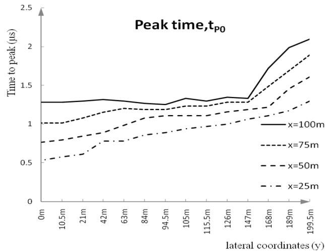
Figure 8: Time taken for induced voltage to peak from lightning instance
