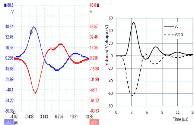
Figure 6: Induced voltages measured (left) and estimated  $x=50\text{m}$ ,  $y=137\text{m}$  by calculation (right). (Coordinates based on Fig. 4)
