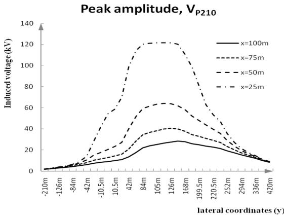
Fig. 7. Peak induced voltages calculated for the other end of the overhead conductor
