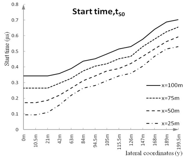
Figure 7: Time taken for induced voltage to appear from lightning instance
