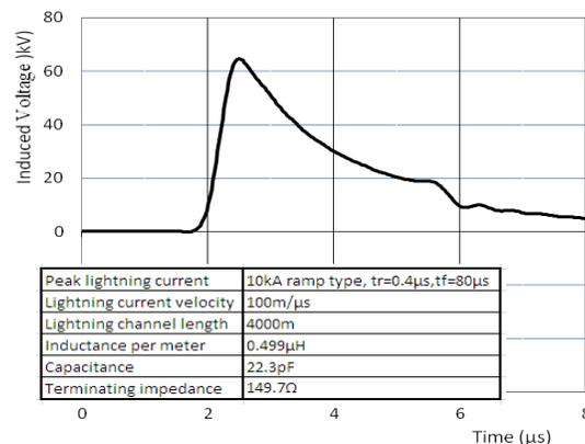
Fig. 4. Induced voltages at both ends of an impedance matched 1km overhead conductor
