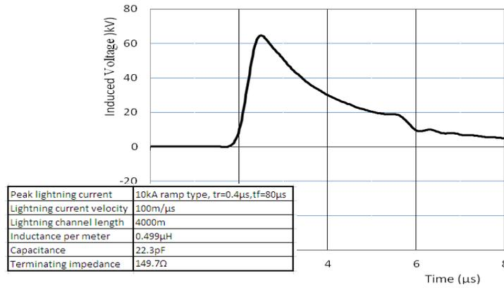
Fig. 2. Induced voltages at both ends of an impedance matched 1km overhead conductor due to 10kA peak current ground lightning 50 meters away equidistant to both ends with input parameters included.
