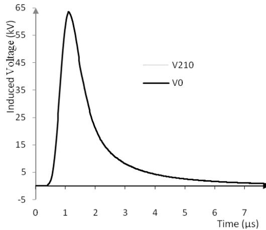
Fig. 9 Induced voltages at both ends with ground lightning strike coordinates of  $(x=50, y=105)$ m.
