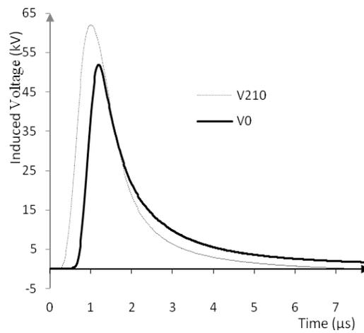
Fig. 10 Induced voltages at both ends with ground lightning strike coordinates of  $(x=50, y=147)$  m.
