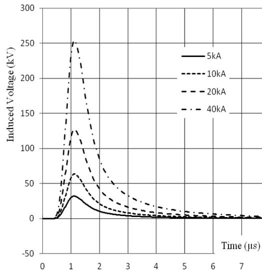
Fig. 14. Calculated induced voltages with varying peak lightning base current
