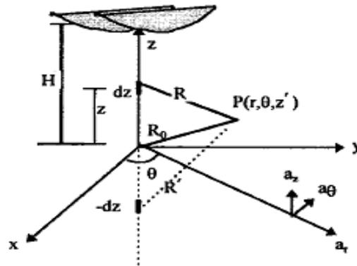
Figure 1: Geometry of a model nearby lightning used in the vertical and horizontal electric fields computation at a point above ground
