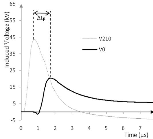
Fig. 11 Induced voltages at both ends with ground lightning strike coordinates of  $(x=50, y=210)$  m.
