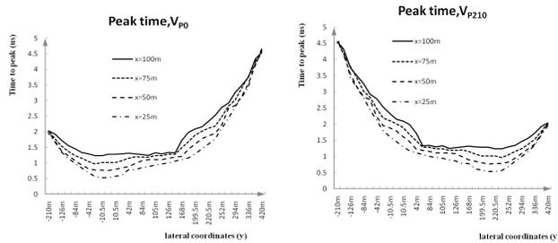
Figure 9: Time taken for induced voltage to peak at the first end of the overhead conductor, (left) and the other end, (right) from lightning instance
