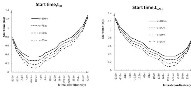
Figure 8: Time taken for induced voltage at the first end of the overhead conductor, (left) and the other end, (right) to appear from lightning instance
