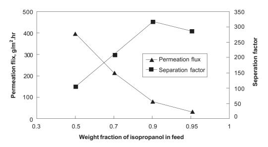
Figure 4 Effect of isopropanol weight fraction in feed on the permeation flux and separation factor
