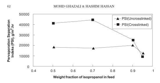
Figure 5 Perporation separation index (PSI) of the uncrosslinked and crosslinked membranes
