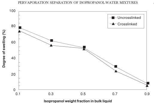
**Figure 1** Degree of swelling versus isopropanol weight fraction in bulk liquid (20 min crosslinking time. Temperature 30°C)
