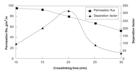
**Figure 3** The pervaporation data of the crosslinked membranes as a function of crosslinking time. Feed isopropanol concentration: 90 wt%
