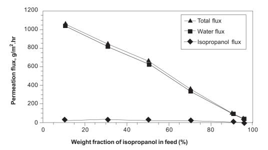
**Figure 2** Effect of feed concentration on the individual permeation flux for the unmodified chitosan membrane (Temperature: 30°C)
