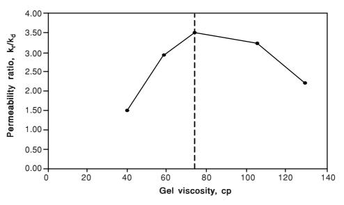
Figure 6 Effect of gel viscosity on the permeability ratio
