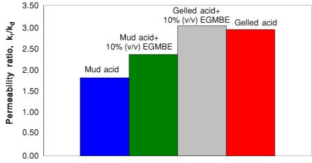
Figure 4 Permeability ratio for different acid systems
