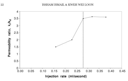
**Figure 5** Effect of injection rate on the permeability ratio
