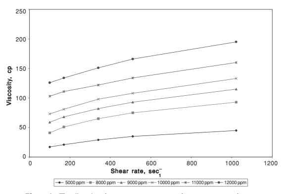
Figure 3 The effect of xanthan gum concentration on gel viscosity at various shear rates
