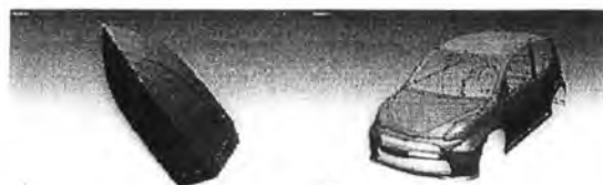
Fig. 12: Curves fitting on 3D models for NURBS surface preparation.
