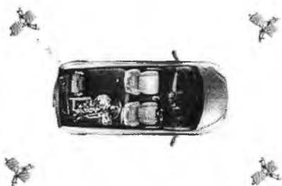
Fig. 9: Faro Photon 80 setup at four different stations with 7m from object.
