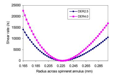
**Figure 7** Shear rate profiles in spinneret at low and high dope extrusion rates with dope solution: 25% CA, 45% acetone and 30% formamide (ratio of acetone to formamide = 1.5)
