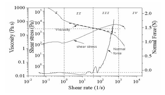
**Figure 3** Flow curve with normal force at 25°C for 27%CA, 36.5% acetone and 36.5% formamide (Ratio of acetone to formamide =1)
