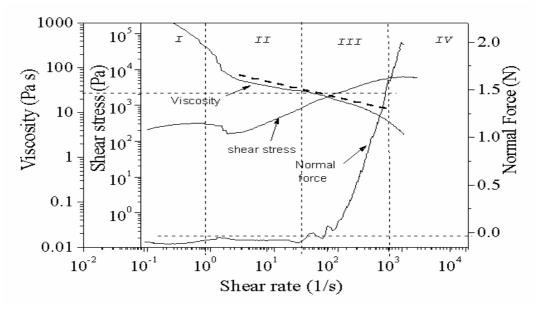
**Figure 4** Flow curve with normal force at 25°C for 27%CA, 43.8% acetone and 29.2% formamide (Ratio of acetone to formamide = 1.5)
