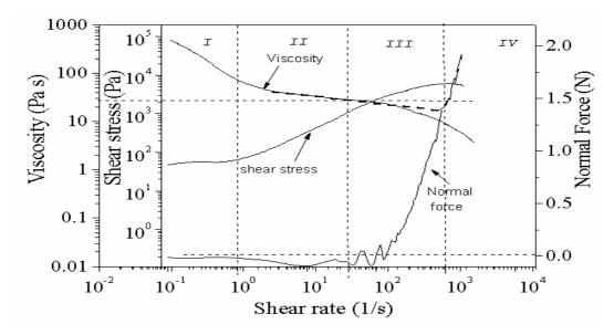
**Figure 1** Flow curve with normal force at 25°C for 25% CA, 37.5% acetone and 37.5% formamide (Ratio of acetone to formamide = 1)
