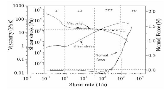
**Figure 2** Flow curve with normal force at 25°C for 25%CA, 45% acetone and and 30% formamide (Ratio of acetone to formamide = 1.5)
