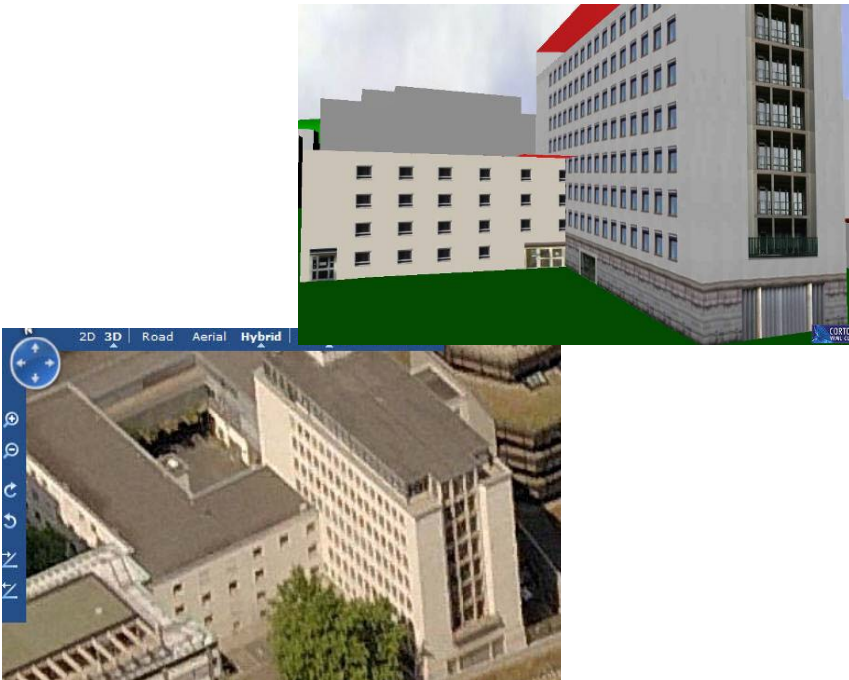
Figure 7: Comparing generated model of one of the buildings of University of Stuttgart with bird view option of Microsoft Virtual Earth.
