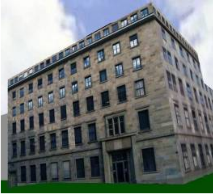
Figure 1: Mapping the images after rectification, obstacles removal and radiometric adjustment on the light weighted geometry of 2 nd building of University of Applied Science in Stuttgart in VRML 2.0
