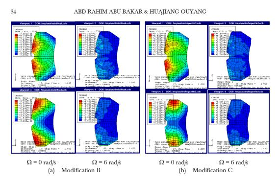
Figure 11 Interface pressure distribution at the piston pad (upper) and the finger pad (bottom)
