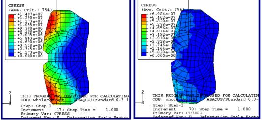
**Figure 8** Contact pressure distribution at finger pad for the original disc brake at speeds of  $\Omega = 0$  rad/s (left) and  $\Omega = 6$  rad/s (right)
