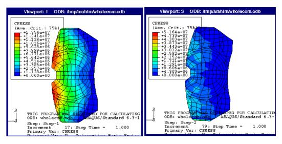
**Figure 7** Contact pressure distribution of piston pad for A4 model at speeds of  $\Omega = 0$  rad/s (left) and  $\Omega = 6$  rad/s (right)
