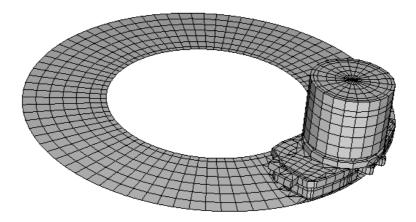
Figure 2 FE model with pad, piston and rigid surface
