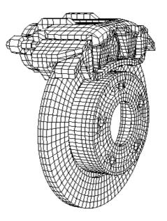
Figure 1 Finite element model of the disc brake
