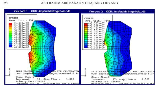
**Figure 5** Interface pressure distribution for model A2 at speeds of  $\Omega = 0$  rad/s (left) and  $\Omega = 6$  rad/s (right)
