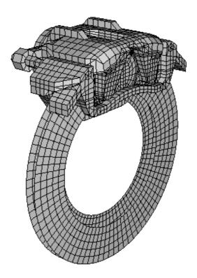
Figure 4 Rigid surface with complete disc brake model
