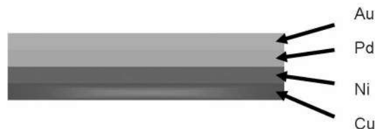
Figure 1 The deposition layers of ENEPIG surface finish
