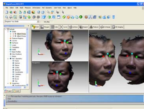
Figure 3: Registration process using image from laser scanner
