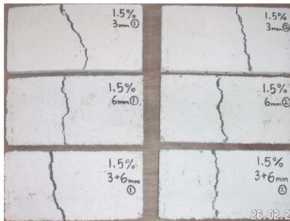
Fig 6. Failure pattern of cement composites containing 1.5% fibers
