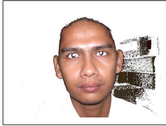
Figure 3.2(b) – Detected human face using only CrCb color space.
