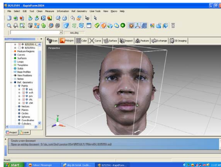
Figure 4: The laser scan data including the 3-D points landmarks in RapidForm software
