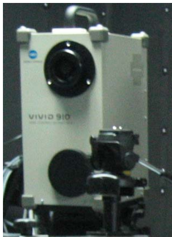
Figure 1: VIVID 910 ( Laser Scanner)
