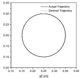
Figure 10 The Trajectory of the Arm in the Last Two Cycles (no disturbance)
