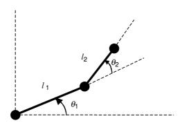
Figure 5 A Representation of a Rigid Two-Link Planar Arm
