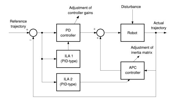
Figure 1 Mechanism of the Proposed Control Scheme
