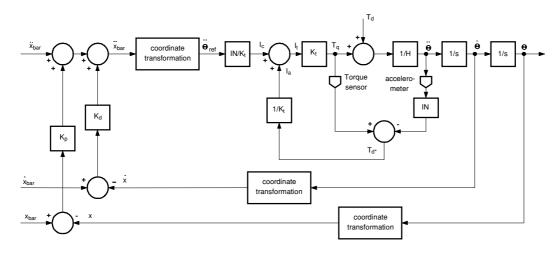
Figure 2 The AFC Scheme Applied to a Robot Arm
