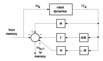
Figure 3(ii) A PID-type Learning Algorithm
