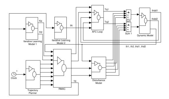
Figure 6 A SIMULINK Representation of the Control Scheme
