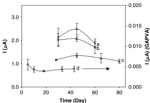
**Figure 2.** Stability of GOD immobilized in different types of membrane: (a) TMOS-PVA hybrid membrane; (b) FTPVA membrane; (c) Al-PVA hybrid membrane; (d) GAPVA membrane. Current response was measured at +0.7 V versus Ag/AgCl upon 5 mmol<sup>-1</sup> glucose addition in phosphate buffer, pH 6.0. The curve for GAPVA is shown at a different scale from the rest.
