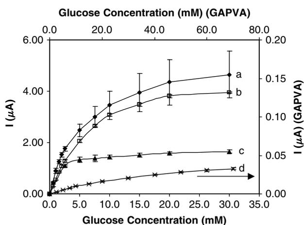
**Figure 3.** Calibration curves of GOD immobilized in different types of enzymatic layer: (a) TMOS-PVA hybrid membrane; (b) FTPVA membrane; (c) Al-PVA hybrid membrane; (d) GAPVA membrane. Current response was measured at +0.7 V versus Ag/AgCl upon 5 mmol L<sup>-1</sup> glucose addition in phosphate buffer, pH 6.0. The curve for GAPVA is shown at a different scale from the rest.
