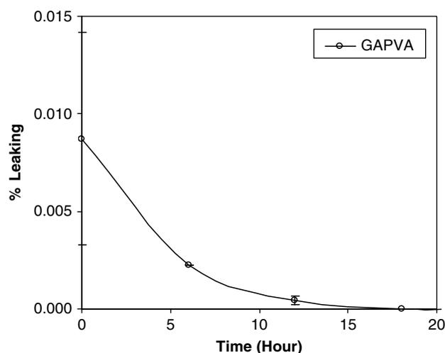
**Figure 1.** Enzyme leakage profile of GOD immobilized in GAPVA membrane. Enzyme activity was determined using a GOD–HRP coupling colourimetric method.
