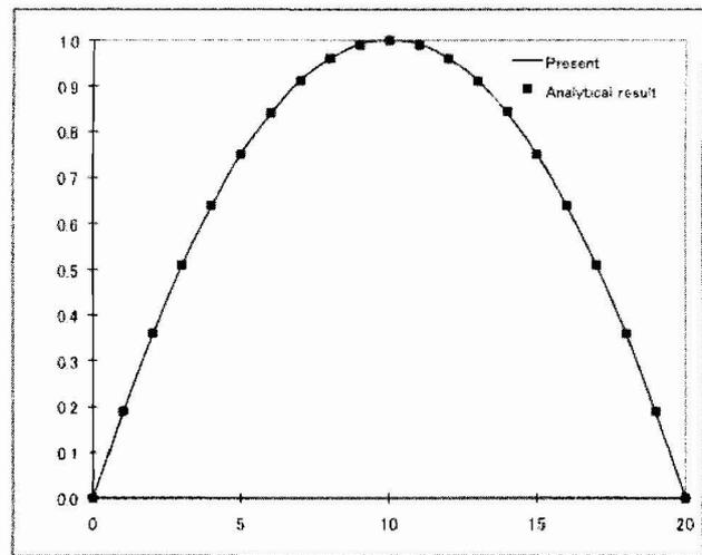
Fig. 2 Comparison of results between LB scheme and analytical solution.
