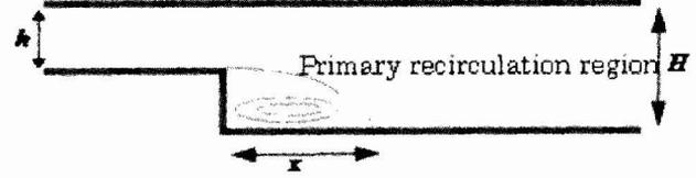
Fig. 3 Sketch of expansion channel flow.
