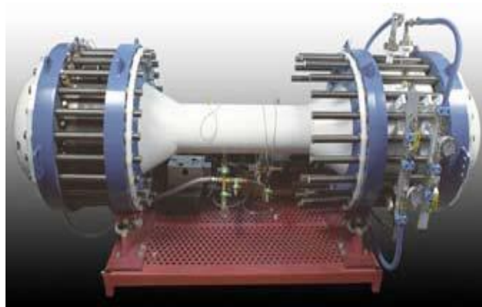
Figure 1.1.2: Standing-wave thermoacoustic refrigerator (Triton: Shipboard Thermoacoustic Cooler, 2005).
