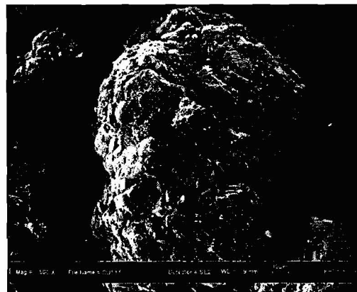
Figure 7 Particles distribution and size (0.018 mm) for Copper catalyst
