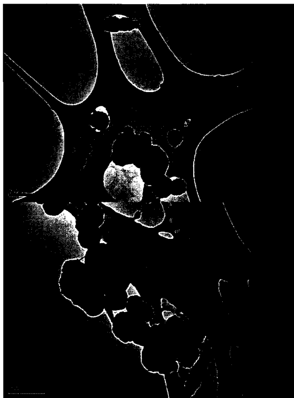
Figure 1 TEM micrographs of geranium oil loaded solid lipid nanoparticles consisting of stearic acid 5% (w/w), Tween 80 and soy lecithin 0.5% (w/w) and dichloromethane 15% (w/w)
