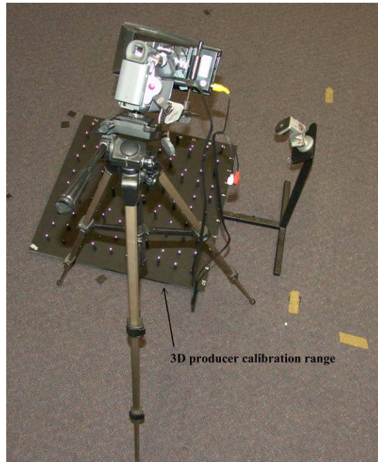
Fig 2. A calibration range constructed for the research.
