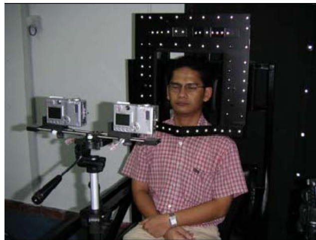
Figure 3: The real stereo camera configuration. The white shining dots are used for camera calibration
