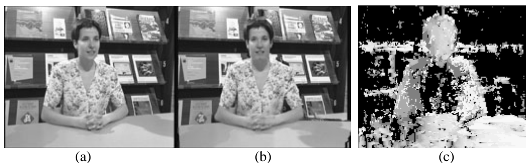
Figure 8: Depth map (a) left image (b) right image and (c) Depth map visualization where the brighter the pixel is the closer to the camera.
