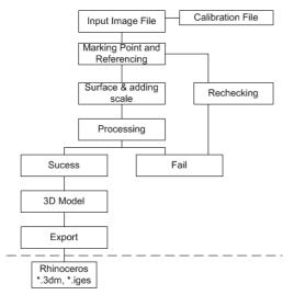
Figure 7: PHOTOMODELER processing and 3D modelling procedure
