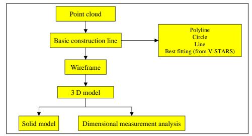
Figure 8: 3D modelling procedure
