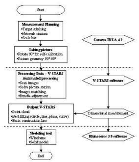
Figure 6: V-STARS measurement procedure
