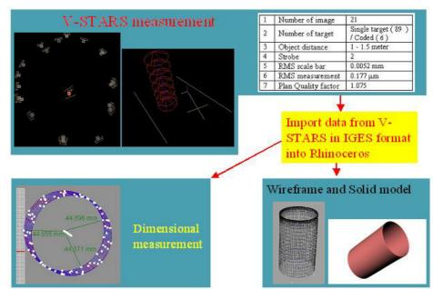
Figure 10: Measurement and 3D modeling of a cylinder
