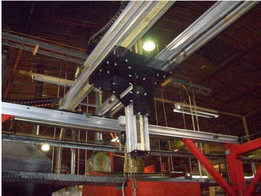
Figure 1.1 : Gantry Robot Structure
