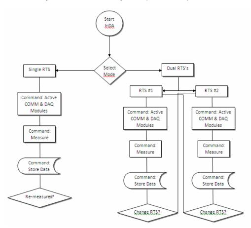
Figure 4. Flowchart for InDA: COMM and DAQ modules.
