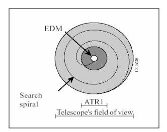
Figure 1. Automatic Target Recognition Concept (Leica Geosystems, 2000)
