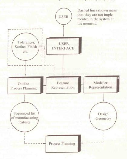
Figure 1: The Main Compenent of the System.
