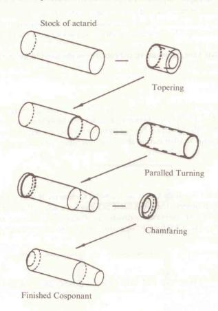
Figure 2: The Feature Representation in DSG Tree Structure.
