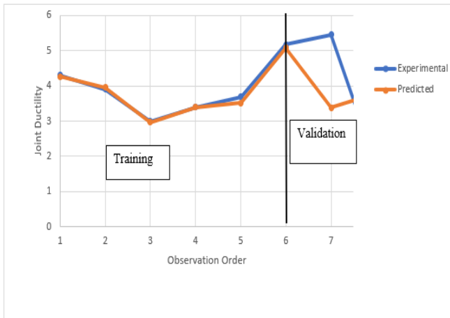
Figure 7 Experimental and predicted joint ductility
