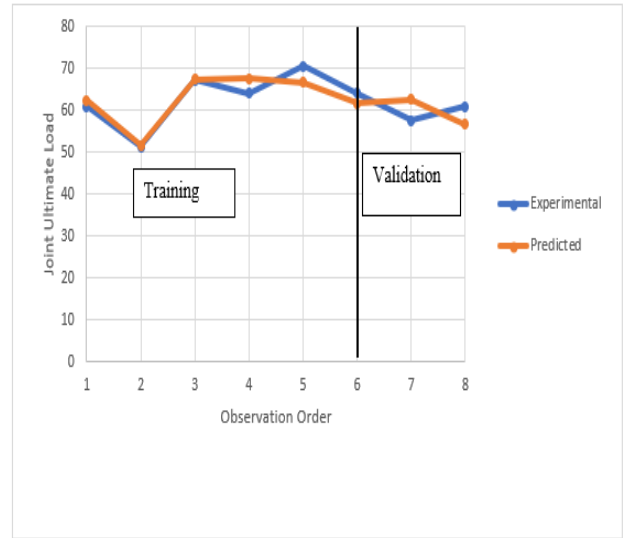
Figure 6 Experimental and predicted joint ultimate load
