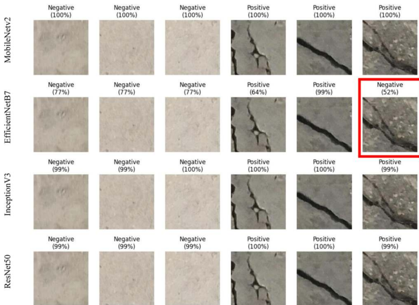
Fig. 5. Sample crack images for with Transfer Learning prediction using CNN models.
