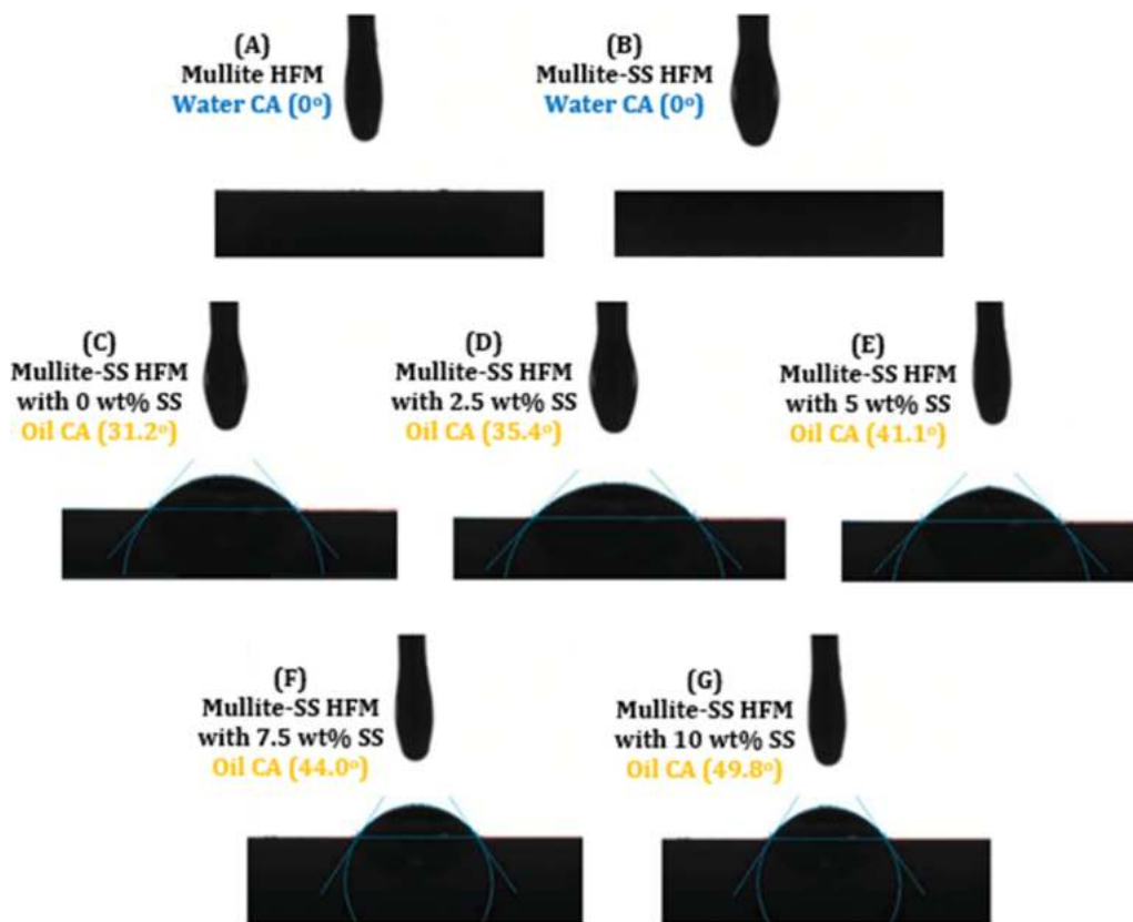
Fig. 19. Water and oil contact angles of mullite-SS HFMs at different SS contents, sintered at 1350 °C.
