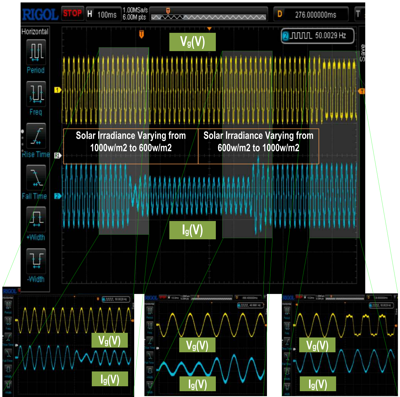
Fig. 14. Processor-in-loop results of v_g(V) & i_g(A) under varying solar irradiance and polluted grid conditions.
