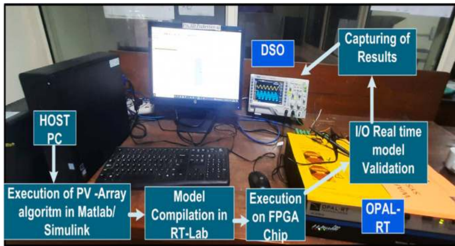
Fig. 12. Experimental implementation of proposed algorithm on OPAL-RT.
