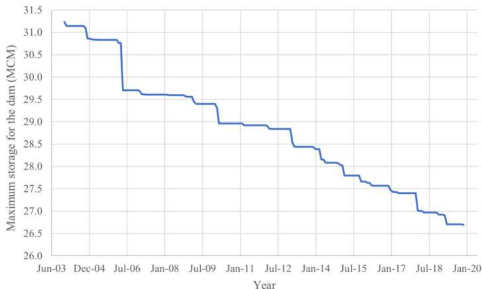
Fig. 7. The effect of sedimentation on the decrease in the actual maximum volume of the reservoir.
