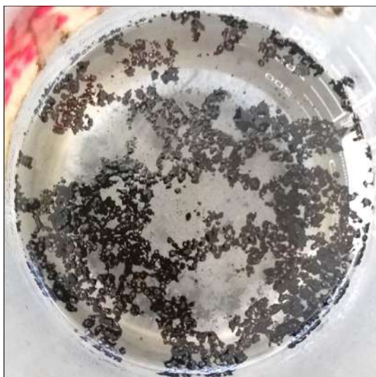
Fig. 5 – A surface to be skimmed during boiling test to avoid re-coating.
