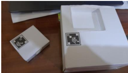
Fig. 13. Printer ZQ300 cardboard mock up
