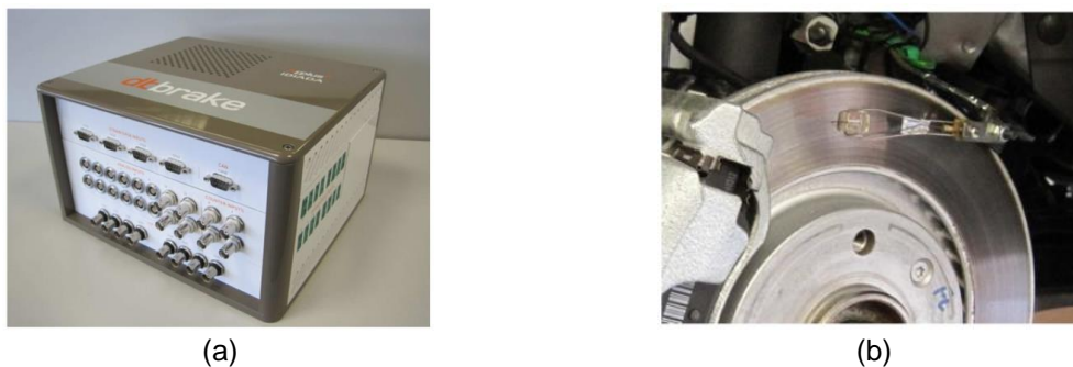
FIGURE 20: dbBrake Noise Evaluation Acquisition System by Applus+ IDIADA (Del Sol & Mateu, 2013). (a) dbBrake system; (b) Rubbing thermocouple on the disc surface
