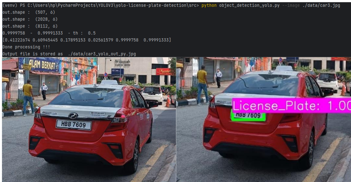
FIGURE 15: Output in the terminal for YOLOv3; Loaded original image; and the output of the image for YOLOv3
