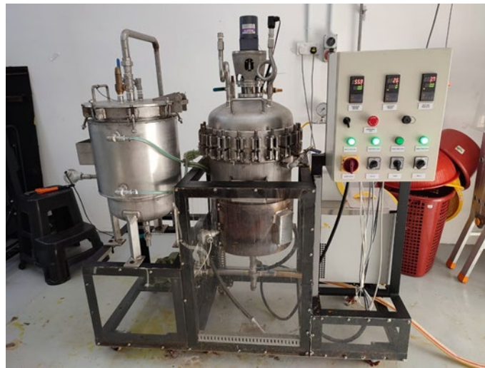
Figure 1: The 70 L subcritical water extractor
