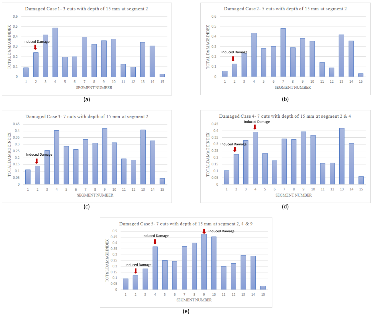
Figure 10 Total damage index plot for (a) Damage case 1 (b) Damage case 2 (c) Damage case 3 (d) Damage case 4 (e) Damage case 5
