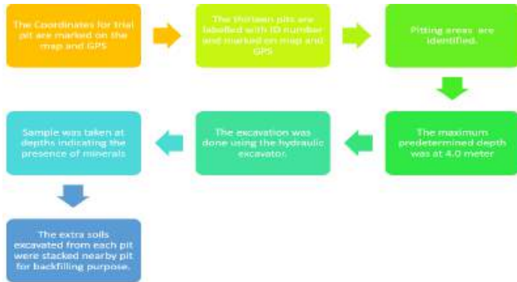
Figure 8: Process flow for Trial Pit sampling
