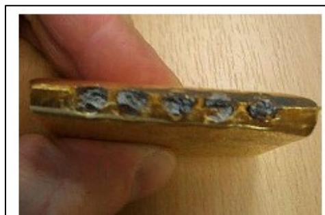
Figure 9. 100 g gold bar plated with tungsten [6]
