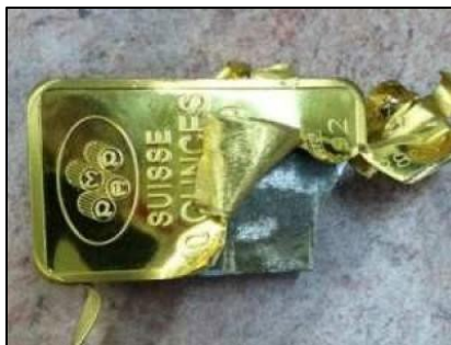
Figure 1. Fake gold bar that contains tungsten [12]
