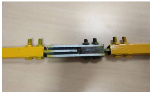
Figure 6. Experimentally tested viscoelastic damper[13].
